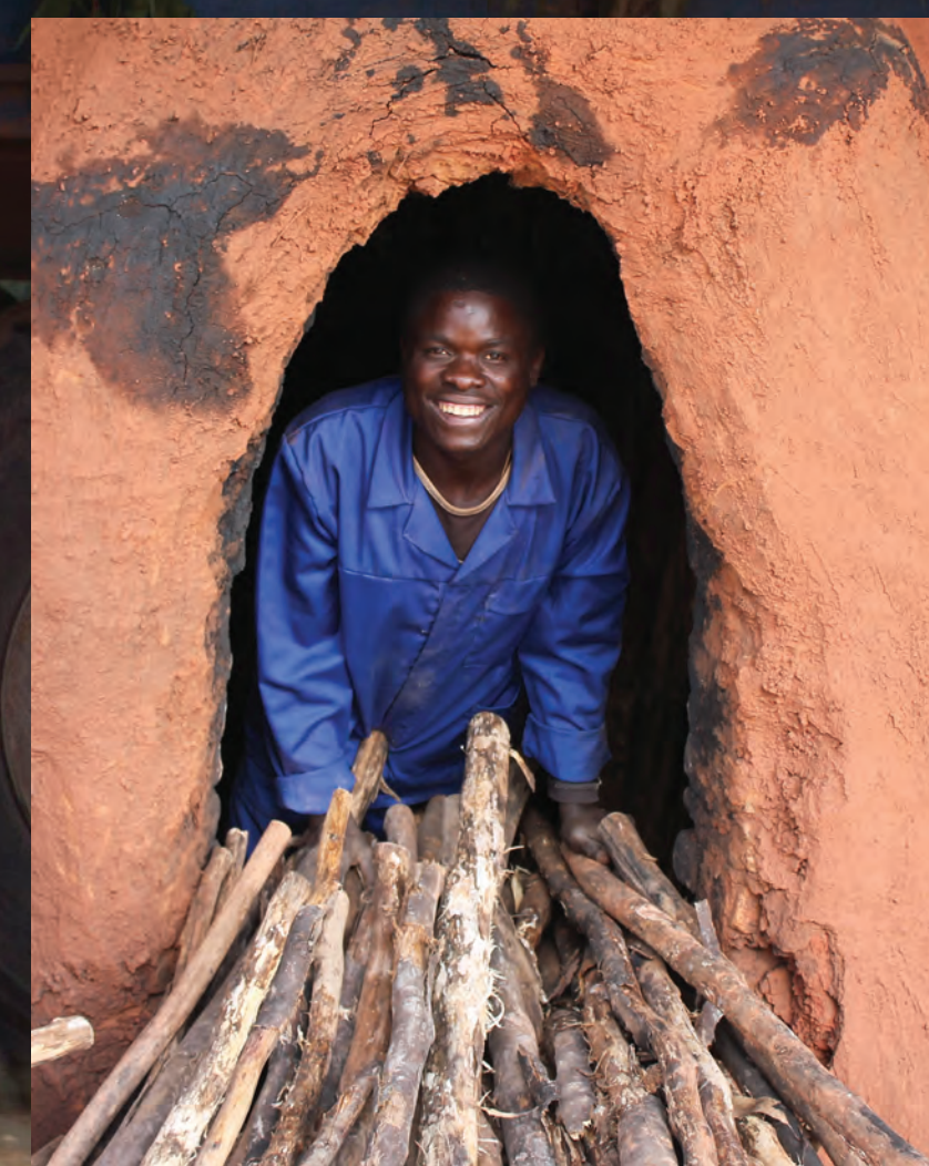
A KHP employee loads a half orange kiln with Corymbia citriodora offcuts to make sustainable charcoal © GINA ALTHOFF/TETRA TECH
